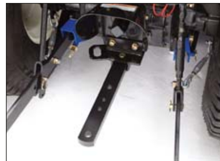
A two-position extendable drawbar is standard equipment to make attaching implements easy.
