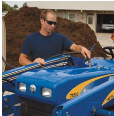
A foldable ROPS is standard on T1500 Series tractors.
